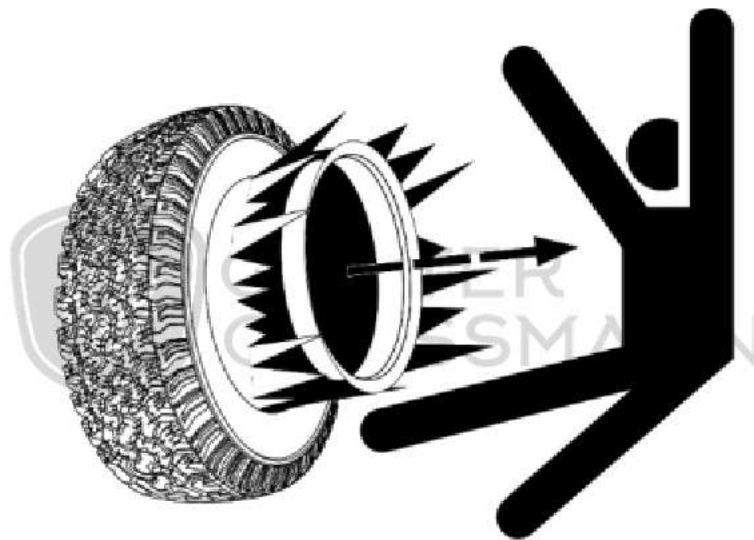
Figure 3-24 Tire explosion risk
