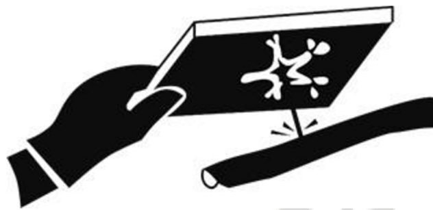
Figure 3-21 Prevent high-pressure oil leaking from small holes
