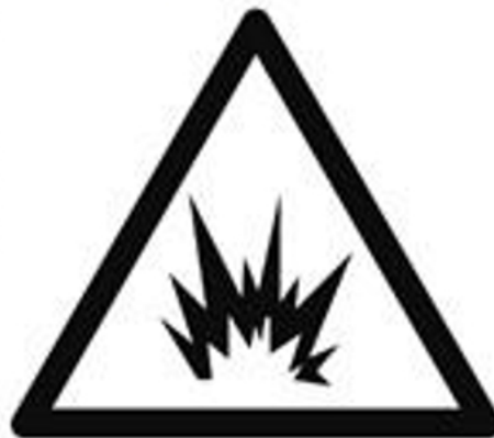
Figure 3-22 Beware of explosion hazard
