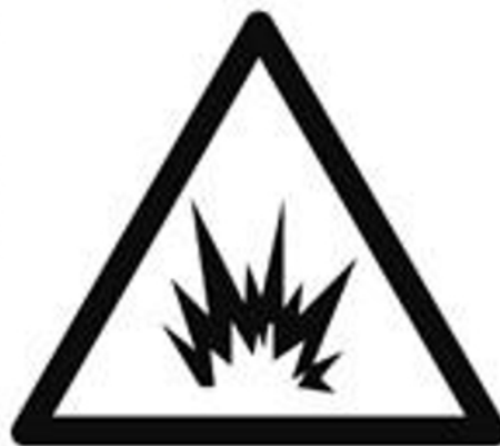
Figure 3-22 Beware of explosion hazard
