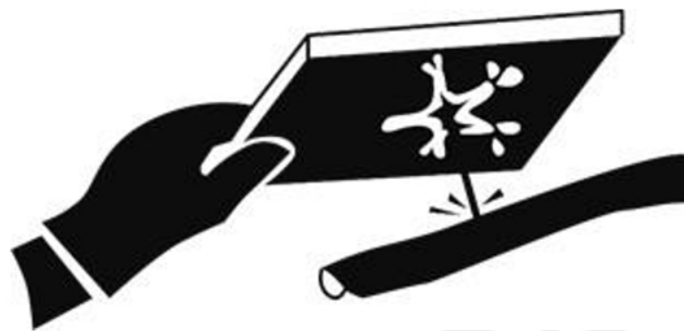
Figure 3-21 Prevent high-pressure oil leaking from small holes
