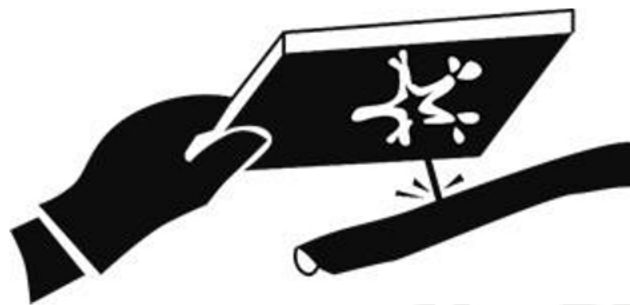
Figure 3-21 Prevent high-pressure oil leaking from small holes
